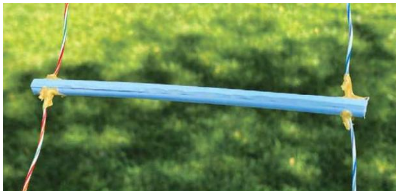
Figure 3 — Feed-line wires are threaded through \frac{3}{64} -inch holes drilled in the spacers, and epoxy is used to hold them in place.
