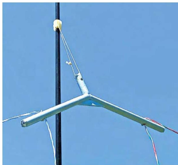
Figure 2 — The top-most spacer is cut from the upper half of a plastic hanger, which provides a convenient antenna attachment point.
